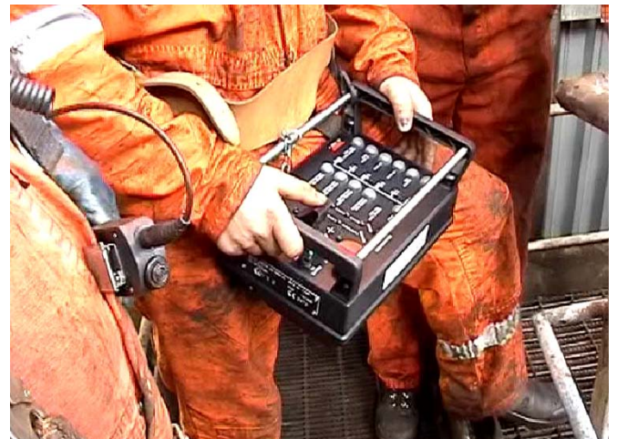
Fig. 7— The portable wireless control panel being used to control the advanced tension frame on Transocean Searcher
